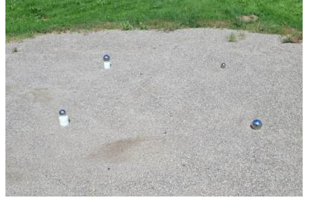
Fig. 3. Reference measurement consisting of four steel spheres above the ground at different heights.
