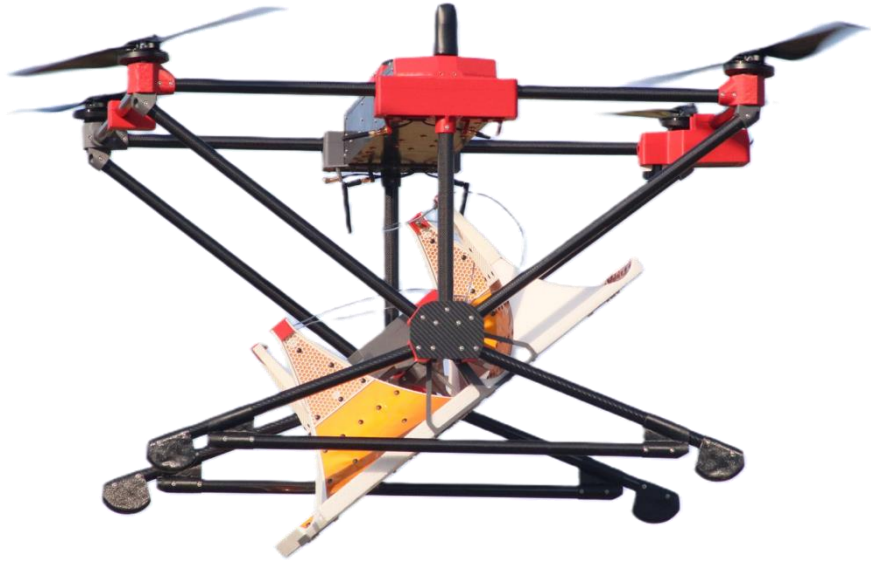
FM-GPSAR UAV Un-manned Aerial Vehicle with Ground Penetration Synthetic Aperture Radar
