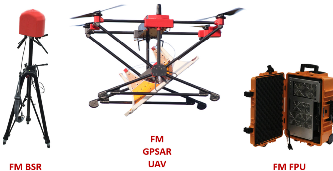
Figure 4 Hardware components of the FM GPSAR system. The ground station is just a commercial notebook and not shown.
